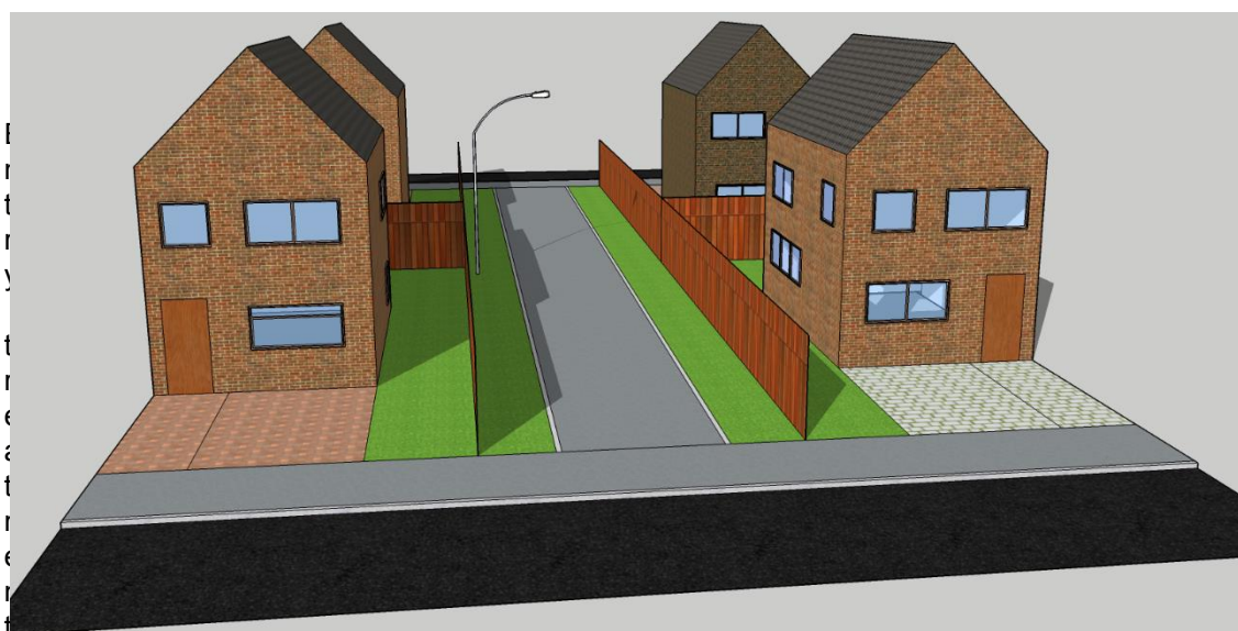
Figure 7 - Typical detail for link path between streets
