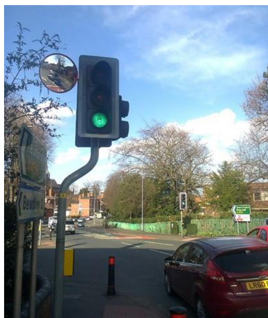
Photo 34 - Example of Trixi Mirror at signalised junction
