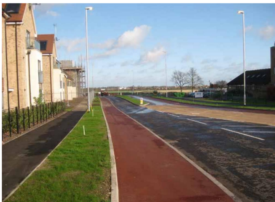
Photo 4 - Example of Hybrid Cycle Track in Cambridge (LTN 01/12)
