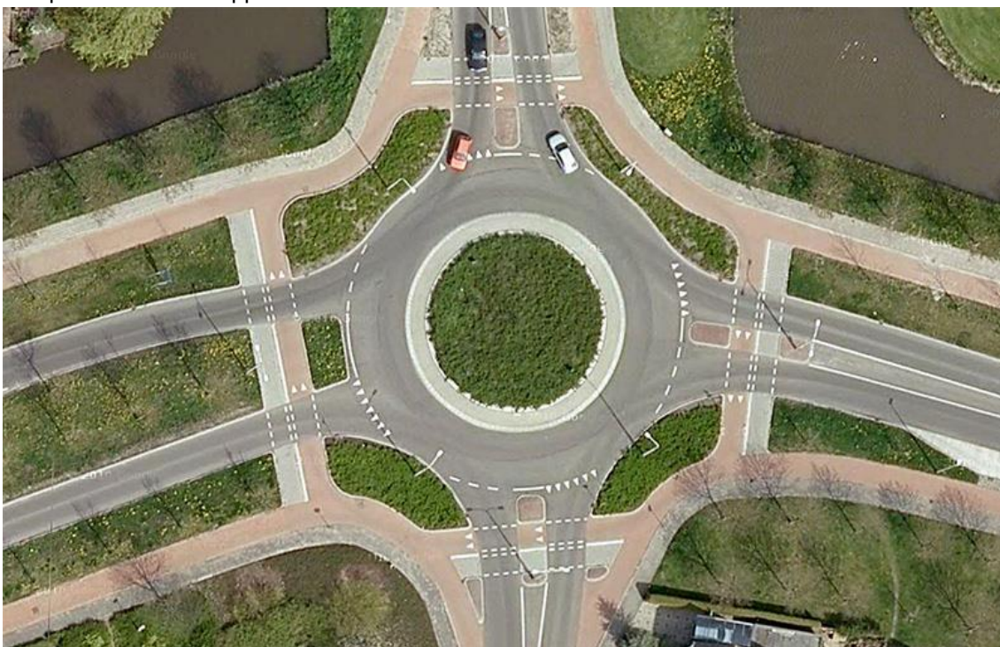
Photo 27 - Example of Dutch style roundabout
