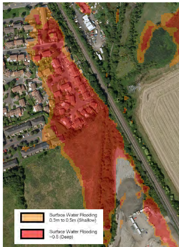
Figure 10-2: Surface Water Flooding in Backworth
