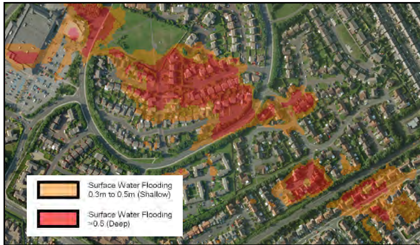
Figure 10-5: Surface Water Flooding in Monkseaton
