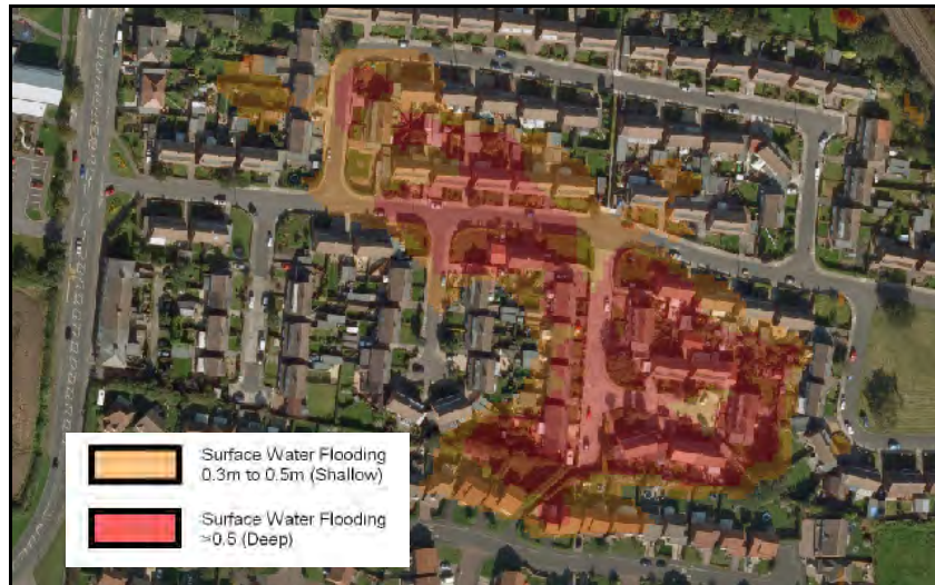
Figure 10-12: Surface Water Flooding in West Moor West
