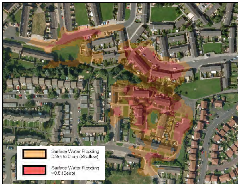
Figure 10-3: Surface Water Flooding in Killingworth
