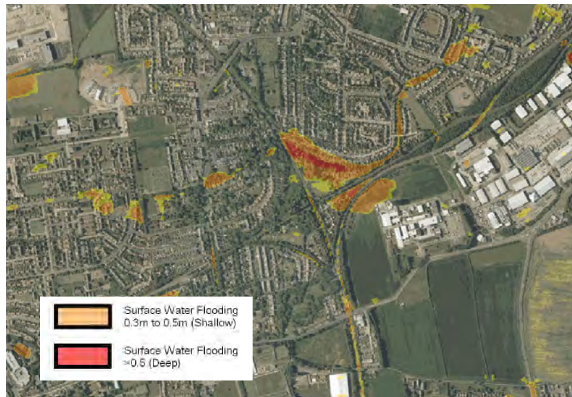
Figure 10-4: Surface Water Flooding in Longbenton
