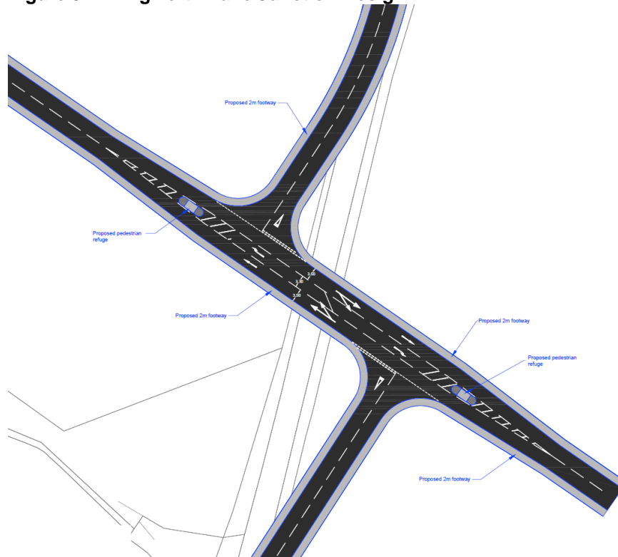
Figure 9 Killingworth Lane Junction Design
