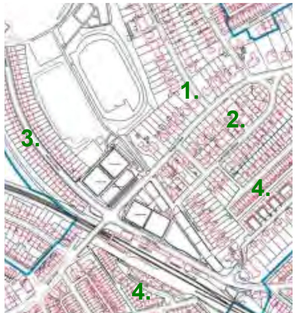
Types of layout in the suburban growth areas. 1: low density detached and semi-detached plots backing onto each other. 2: the same but ratio altered to balance the street scene. 3: linked semis. 4: tighter terraced layouts with back lane access.
