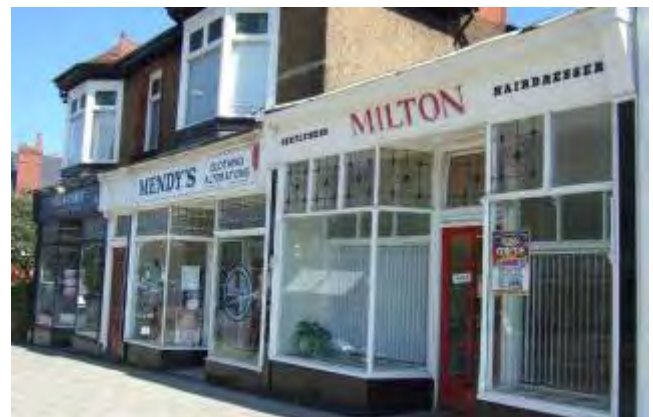
Leaded toplights with painted and textured glass are characteristic
