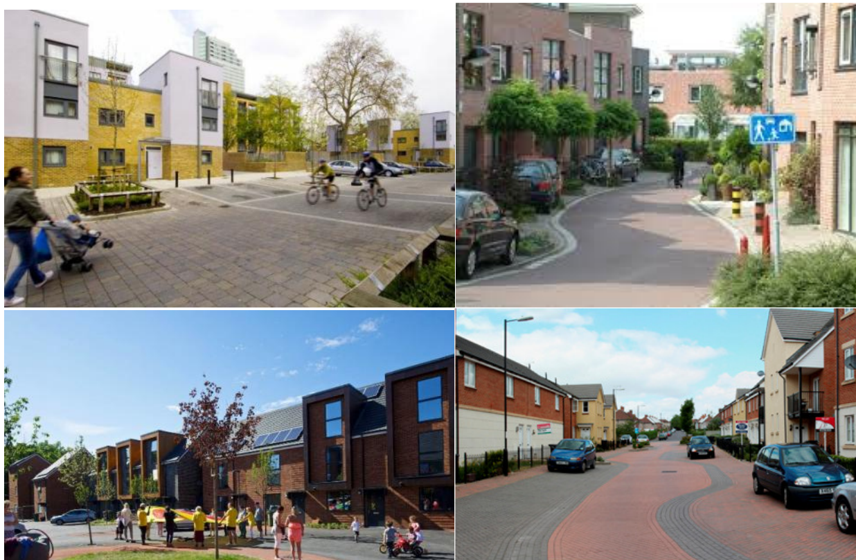
Figure C.5 – Examples of shared space treatment with all modes at the same grade. Shared space aims to minimise the segregation of pedestrians, cyclists and vehicles with a desire to reduce the dominance of vehicles, vehicle speeds, and road casualty rates. This is done by removing features such as curbs, road surface markings, traffic signs, and traffic lights. By creating a greater sense of uncertainty and making it unclear who has priority, drivers will reduce their speed resulting in a safer environment for pedestrians, cyclists and vehicles.
